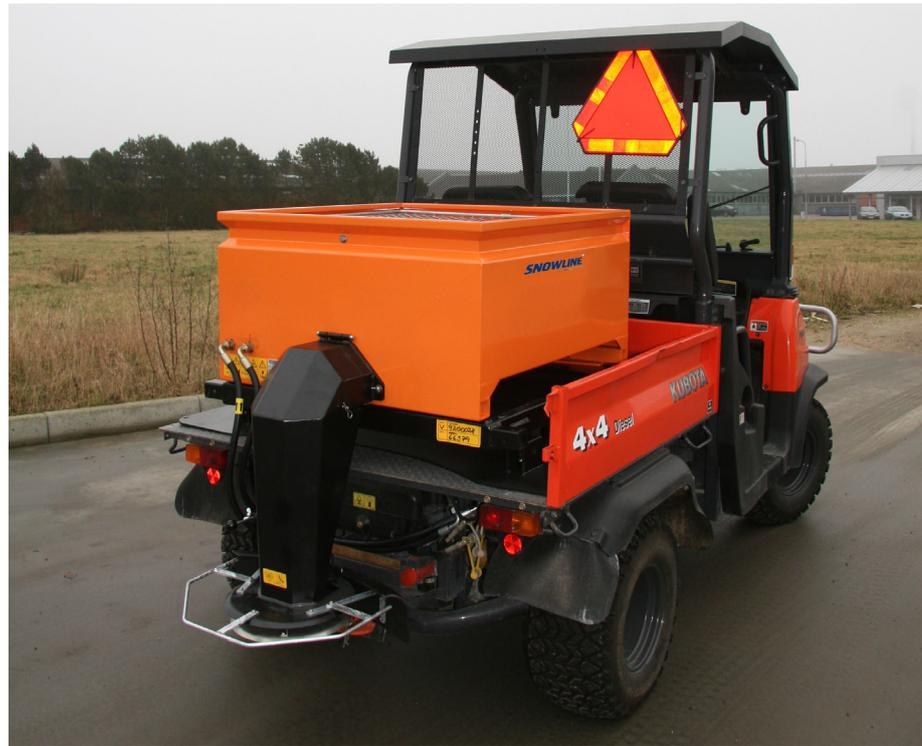
spread symmetry can be moved from right to left. The machine is suitable for a variety of carriers.
